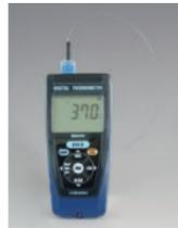
Precise temperature measurement is possible by using a thin sensor with Teflon covering and excellent chemical resistance.
