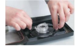
Even when the objective interferes with the bottom of the dish, a spring type buffering mechanism prevents breakage of the dish/objective.
