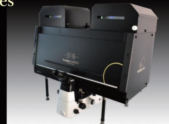
Automatic Thermo-control System (For IVF and basic research)
